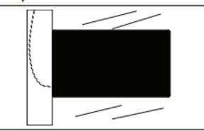
Adhere the backing label to the oposite side of the glass to hide the back of the Surface Mount and iPad.
