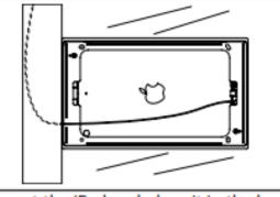
Connect the iPad and place it in the bezel. Attach the bezel to the bracket. Adhere the Surface Mount bracket to the glass close to the channel.
