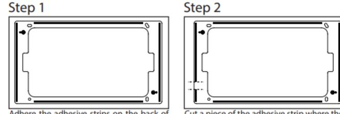
Adhere the adhesive strips on the back of the Surface Mount bracket as shown.
